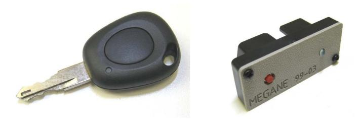
The Megane Reconfiguration Pod (MRP) reconfigures the UCH to immobiliser 'System Type 1', so that the vehicle can be started, and an RPM fitted as a long term fix.
