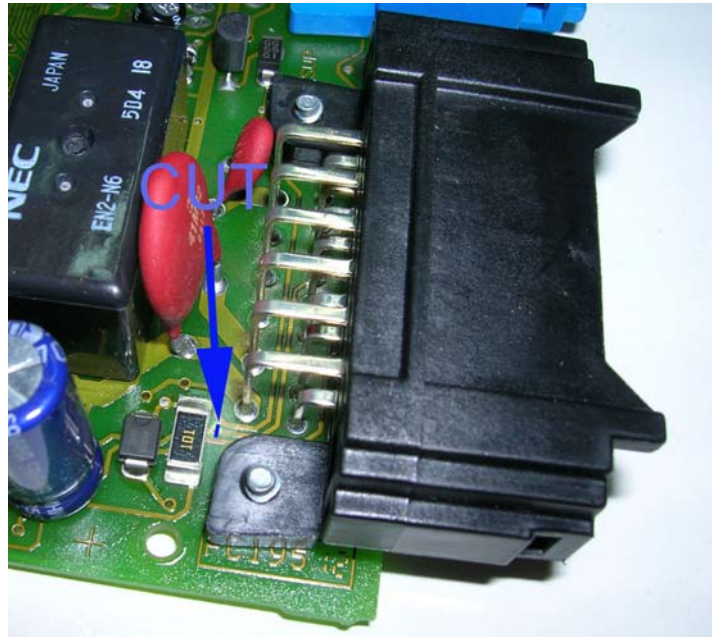
Track to cut, to stop LED from flashing, units with Motorola microprocessor
