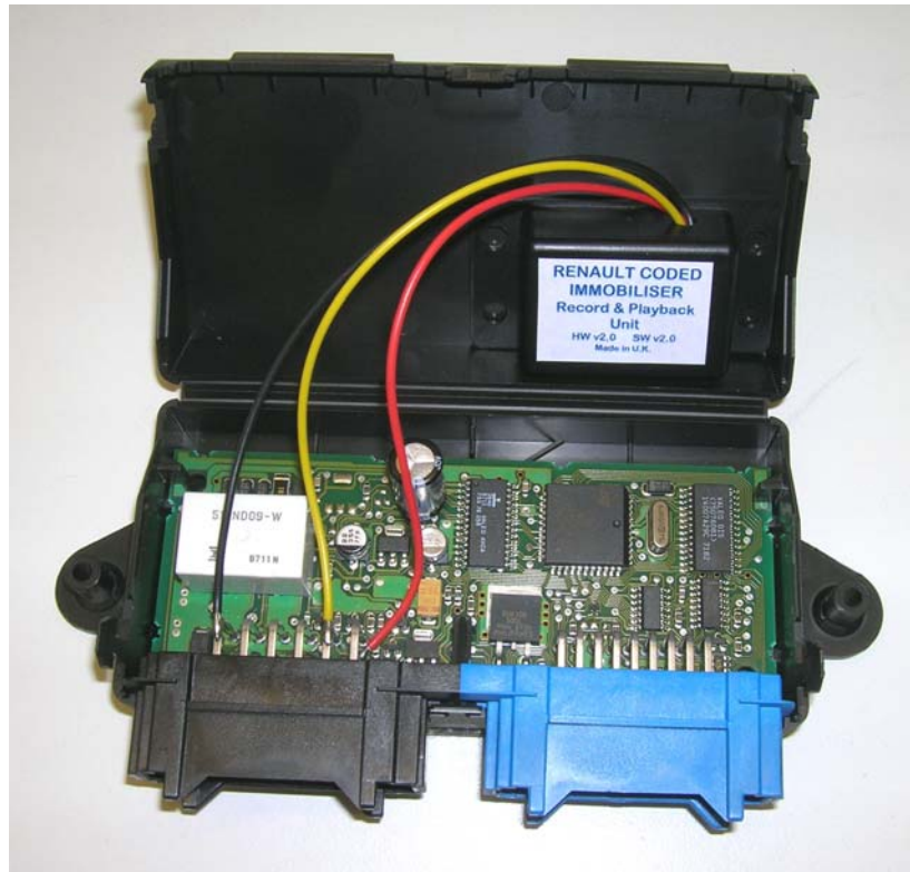
Typical view of an RPM unit, mounted using double sided foam tape
