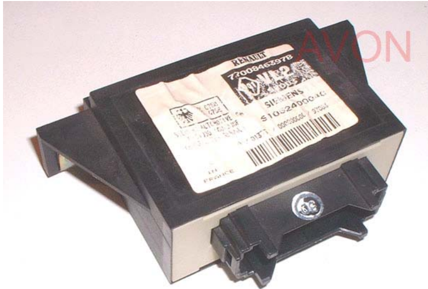
Transponder Only Decoder unit, Motorola 68HC05 Microprocessor
