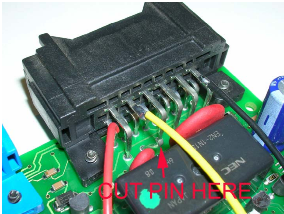
Detailed view, showing soldered connections
