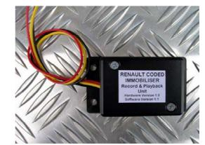
If you can disarm the original immobiliser once, either by entering the over-ride pin, or by substituting components (e.g. a working infra red receiver), it's possible to program the Record and Playback Module without any other specialist tools.
