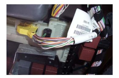
Once the yellow connector has been unplugged, it's possible to slide the black insert out of the yellow housing:
