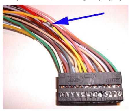
Data: Yellow wire on Record / Playback module to Pin 15 on Yellow way connector (usually an orange wire)
