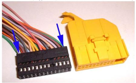
Terminal numbers are moulded into the corners of the black insert, as shown by the blue arrows
