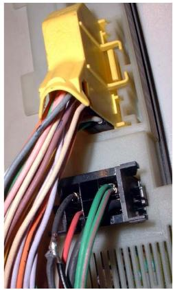
Ignition: Red wire on Record / Playback module to Pin 6 on Yellow 26 way connector (usually a yellow wire)
